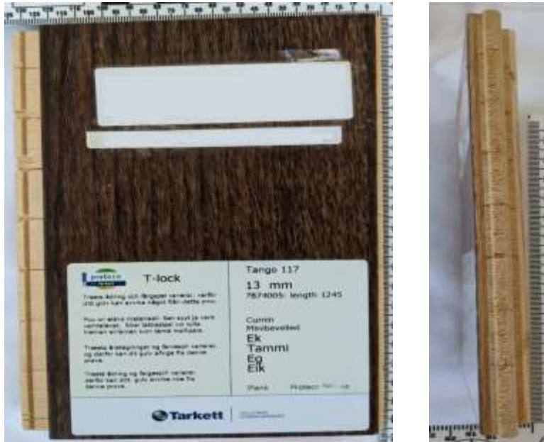
Image 3. Laminate Wood Panel (Battenboard) of Subheading 4412.94 – Photo of a laminate wood panel with one piece laminate sheet face up, battenboard core and laminate sheet back, and a second photo of the laminate wood panel cross section.
