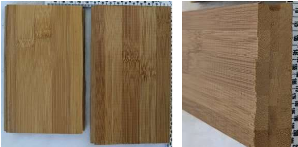
Image 4. Assembled multilayer bamboo flooring panel of Subheading 4418.73 – Photo of a multilayer bamboo panel of two or more strips on the top surface, and a second photo of a cross section of the multilayer panel composed of several assembled strips on each of the top, middle and back layers.
